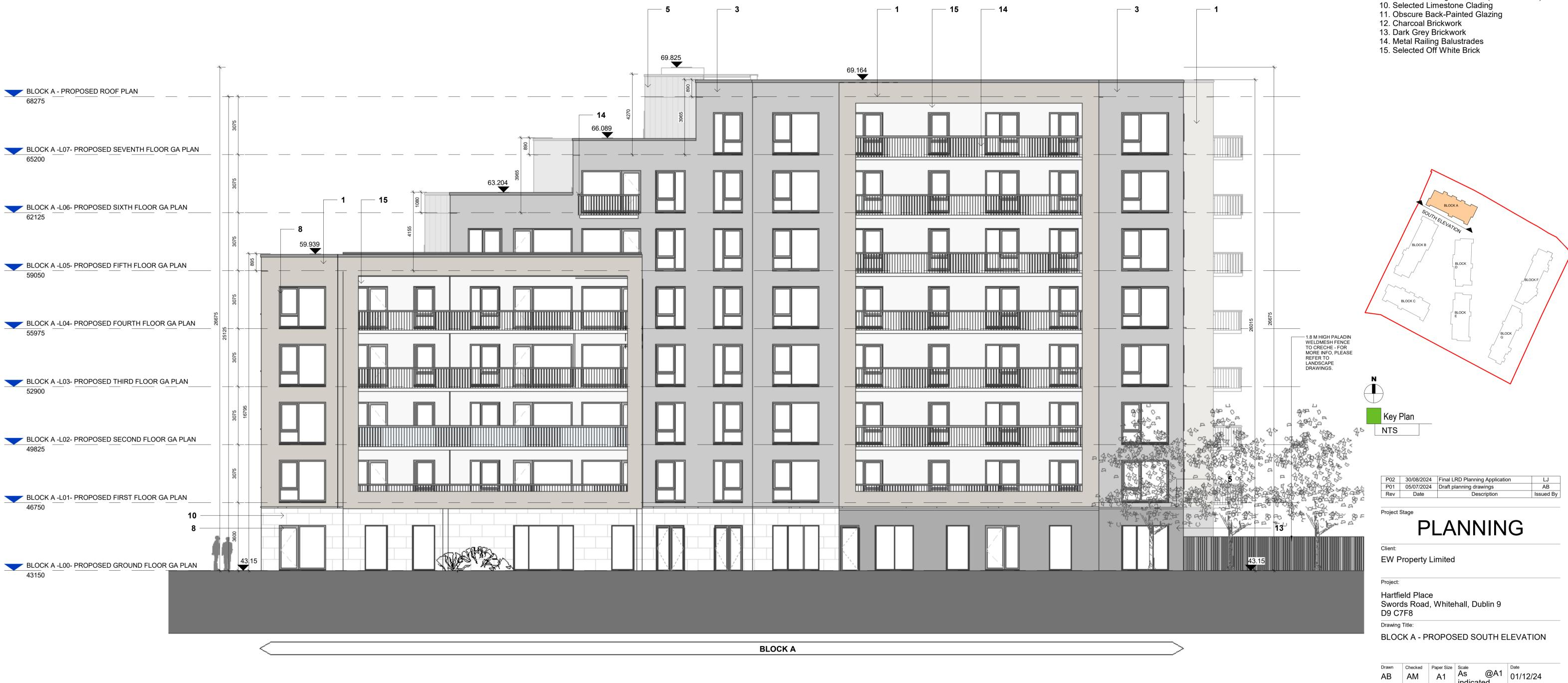
1 BLOCK A - PROPOSED SOUTH ELEVATION 1 : 100
