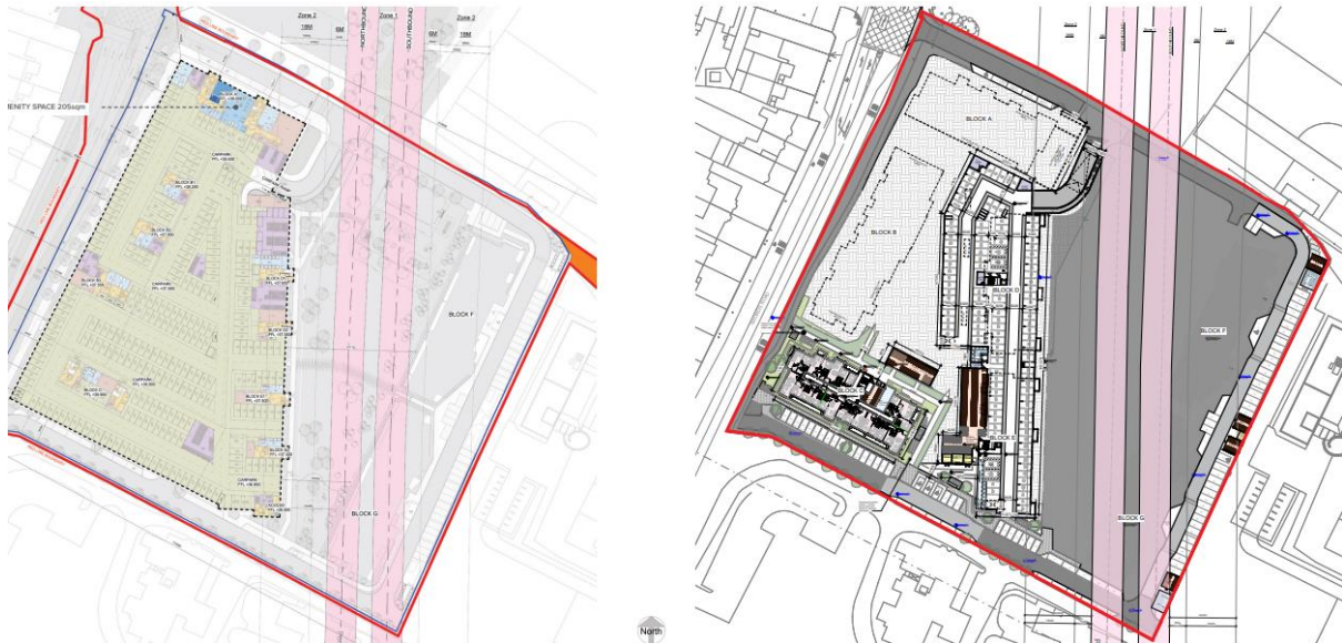
Figure 11 -Permitted basement to the left and Proposed basement to the right
