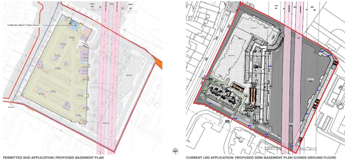
Figure 19- Permitted Basement (left) & Proposed Semi basement (right)
